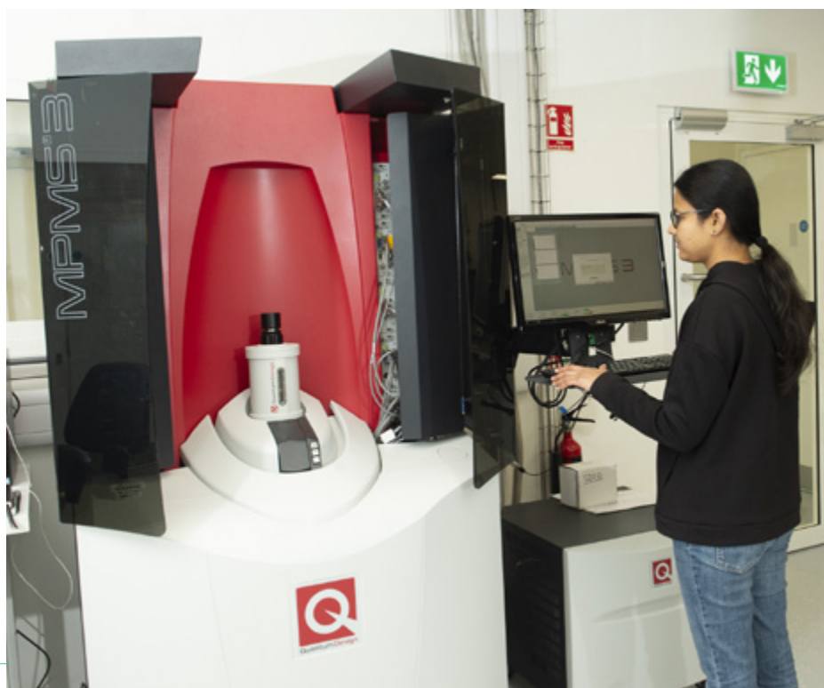
Quantum Design MPMS 3 SQUID (superconducting quantum interference device)
